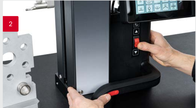
2 The ergonomic thumbwheel and function keys enable operators to easily and quickly position the measuring probe and to start the measurement. For very large workpieces an air bearing, that is activated via keys in the handle, supports the exact positioning of the device.
